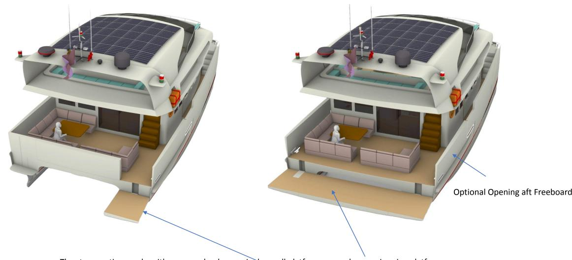
The stern section can be either opened only as a single small platform or as a large swimming platform
