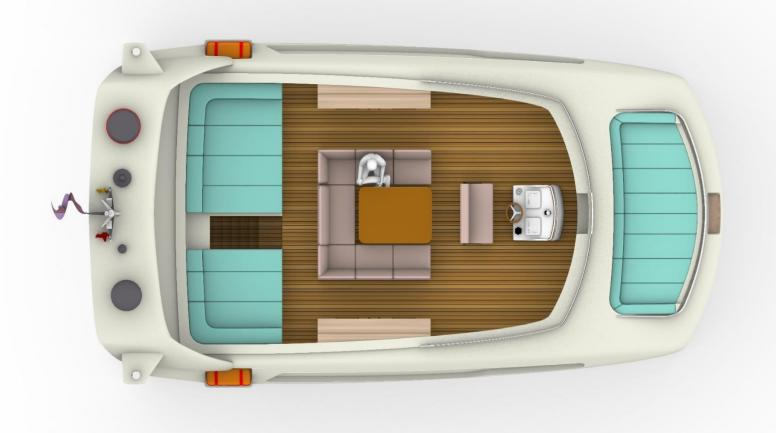
Sun cushions with underneath storage MY Boat 48' Main Deck Features & Options Fender storage Leasure corner with entrance to captains quarters Plenty of additional locker space Day Head Large galley Openable freeboard Storable BBQ **Pilot Station Swimming Platform** 3 cabins with full head/shower
